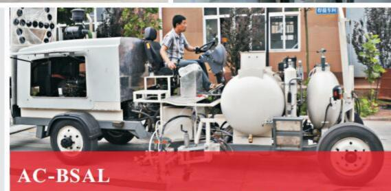
Big Driving-type Cold Paint Airless Road Marking Machine
